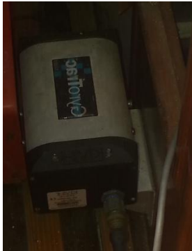
Figure 10 Gyrotrac magnetic gyro compass
