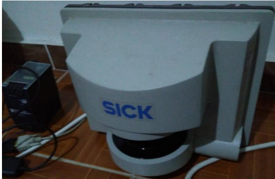
Figure 7 A close image of the sick LMS221 laser measurement system
